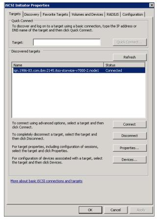
Figure 5-36 iSCSI Initiator target is connected
