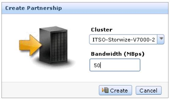
Figure 11-65 Select the remote IBM Storwize V7000 storage system for a partnership
