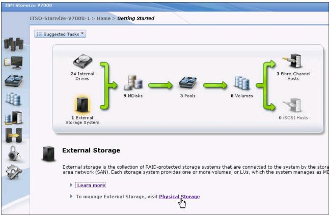
Figure 9-4 Access External panel from Getting Started panel
