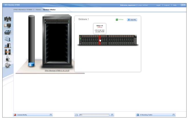
Figure 3-16 System Status screen showing an offline component
