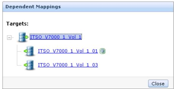
Figure 11-40 FlashCopy mapping dependency
