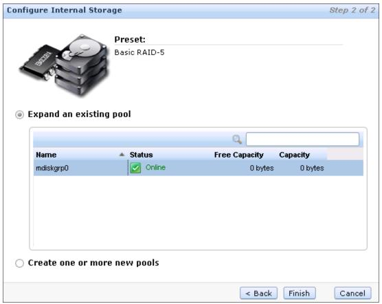
Figure 7-18 Assign new capacity to an existing storage pool
