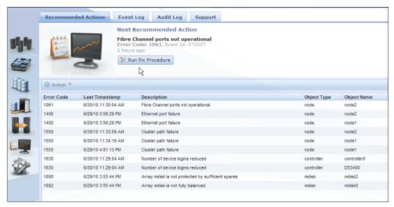
Figure 13-30 Recommended Action: Fibre Channel Ports Not Operational
