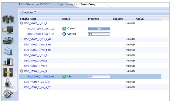
Figure 11-24 New FlashCopy mapping has been created with new target
