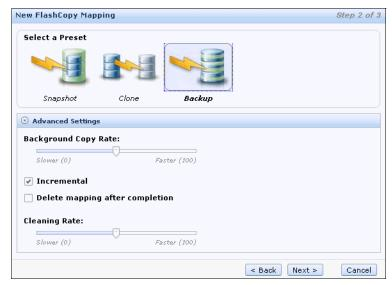
Figure 11-28 Select preset and make your adjustment to the settings
